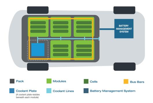
Cells are the basic building block of a battery pack. Within newer packs, cells typically use a lithium chemistry base. There are three major types of cell architecture:
